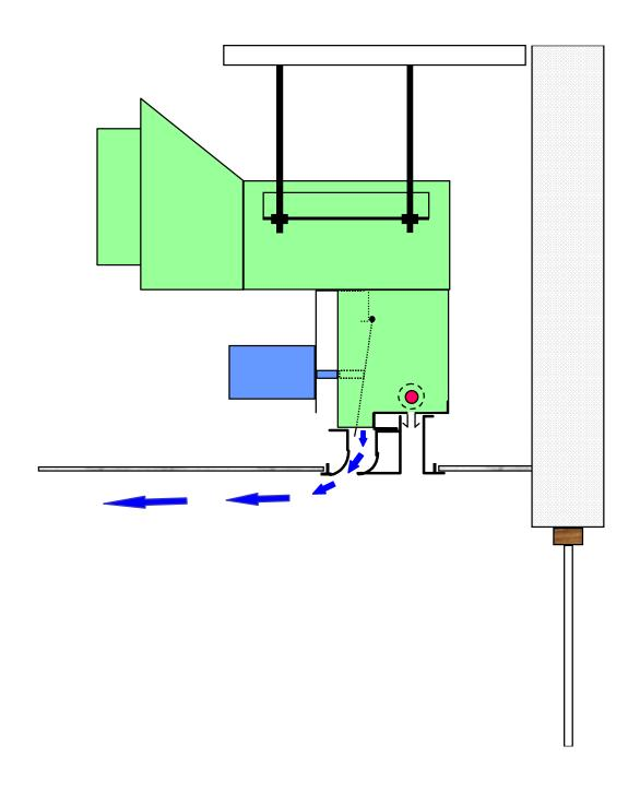
CLM-W1 CONTROPLANE PERIMETER VAV TERMINAL SHOWN IN THE COOLING MODE SUPPLYING AIR HORIZONTALLY ACROSS THE SPACE.
