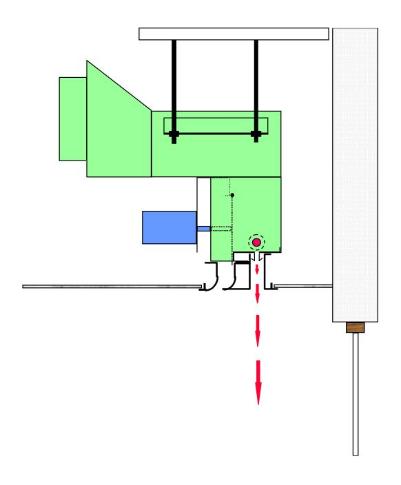
CLM-W1 CONTROPLANE PERIMETER VAV TERMINAL SHOWN IN THE HEATING MODE SUPPLYING AIR VERTICALLY DOWN THE BUILDING'S INTERIOR FACADE.
